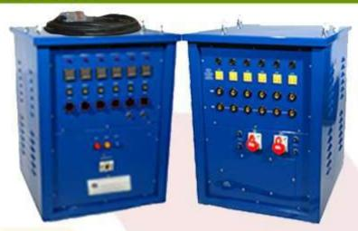
The 50 kVA heat treatment unit has been robustly constructed to provide power to electrical resistance heaters at 60 volts, suitable for site and shop working. The output from the unit is split into six individual heating circuits for temperature control. Each output circuit has 8.3 kW of power, which is sufficient capacity for three standard ceramic pads rated at 2.7 kW and connected in parallel.
