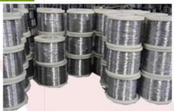
This wire has 37 strands and can be used in our Ceramic Heater Pads and Flexible Insulated Preheaters.
