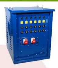
The 65 kVA heat treatment unit has been robustly constructed to provide power to electrical resistance heaters at 60 volts, suitable for site and shop working. The output from the unit is split into six individual heating circuits for temperature control. Each output circuit has 10.8 kW of power, which is sufficient capacity for four standard ceramic pads rated at 2.7 kW and connected in parallel.
