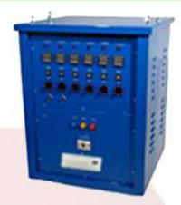
The 73 kVA heat treatment unit has been robustly constructed to provide power to electrical resistance heaters at 60 volts, suitable for site and shop working. The output from the unit is split into six individual heating circuits for temperature control. Each output circuit has 12.1 kW of power, which is sufficient capacity for four standard ceramic pads rated at 2.7 kW and connected in parallel.
