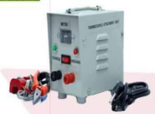
The equipment is suitable for welding Thermocouple wires of different material to steel / alloy steel plate. One terminal is connected to plate by "Earth" magnet, while Thermocouple wire to be welded is being held in "Nose player" and kept in contact with plate. "Weld switch" / Foot switch is used to weld the wire on the plate. Capacitors can be charged to different voltages to get different values of weld current.
